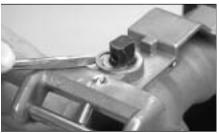
**4.** While pushing the disc up into the body, insert the retaining ring into the slot on the disc stem. With the disc rotated in the half turn position, insert the disc retainer pin tapping with a hammer to insert the oversized grooved end on the pin into the hole in the disc stem. Rotate the disc several times to ensure proper function.
