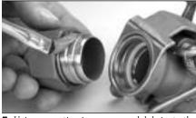
**5.** Using an anti-seize compound, lubricate the spline and spline groove on the swivel body.
