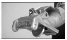
**1.** Remove the adapter cover, side panels, locking cap and the main seal (See Kits I and K for instructions).
