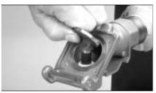
**3.** With the disc rotated a half turn, remove the retaining ring from the top of the disc stem and pull the disc out from the coupler body.
