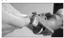
**5.** With the disc rotated a half turn or 180° from the closed position, insert the disc retaining pin into the stem hole. Use a hammer and lightly tap the pin into position.
