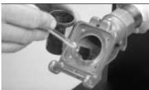
**2.** Apply an anti-seize compound into the stem hole in the coupler body. Anti-seize should **not** be present in the stem seal area. Apply a light lubricant to the stem seal and the stem seal area of the coupler body.
