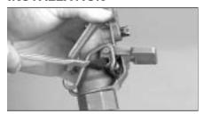
**1.** Reassemble the locking bar and locking arm. Ensure proper position. Lubricate the holes in the locking arm with an anti-seize compound.
