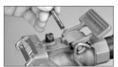
**2.** Remove the locking arm standoff. Remove the locking arm spring and locking bar springs.
