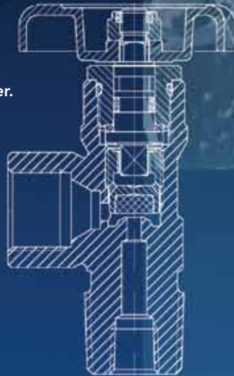
Part number A510-6-0 designed with CGA510 outlet for acetylene service, 3/4 NGT Inlet for steel cylinders, no safety device.
