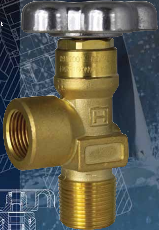
Part number A510-6-0 designed with CGA510 outlet for acetylene service, 3/4 NGT Inlet for steel cylinders, no safety device.
